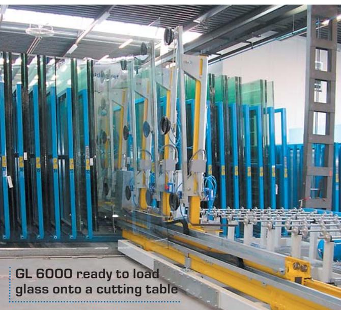
GL 6000 ready to load glass onto a cutting table
